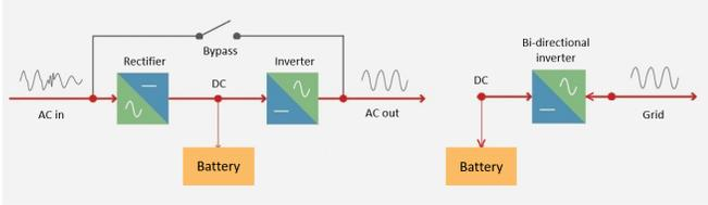
Fig. 2: Different connections of battery to grid
