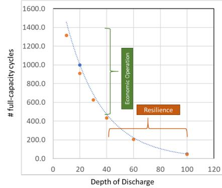
Fig. 4: Relationship between DoD and the number of cycles for each cell
